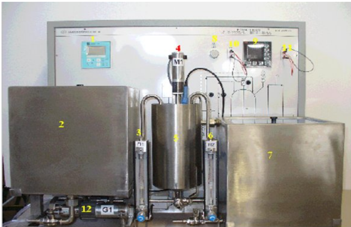
Figure 1.3 pH control system
