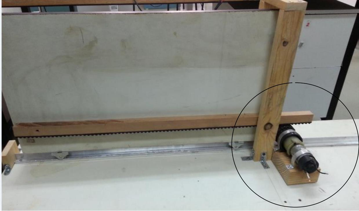
**Figure 36: picture of motor connected to the door.**
