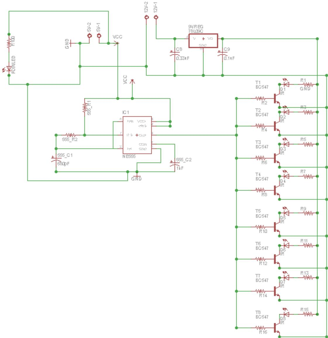
Figure 0-4: 8-IR Led connection, Transmitter
