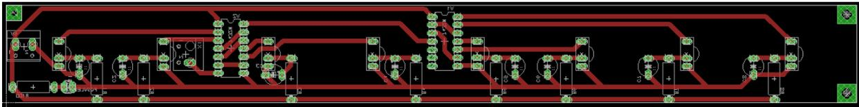
Figure 0-7: The Printed Circuit Design For TSOP, Receiver
