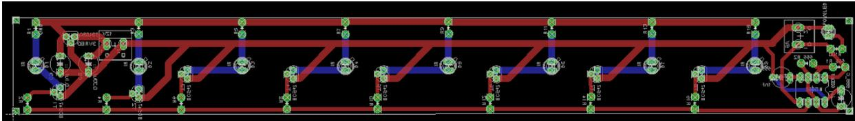
Figure 0-6: The Printed Circuit Design For IR Led, Transmitter
