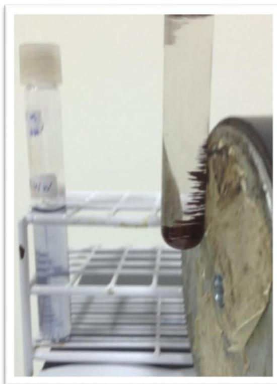
Figure 3.1: A photograph of dye adsorptive removal from real textile wastewater sample by magnetic nanoparticles. The photograph was taken by Nidal Marie in May 2013.
