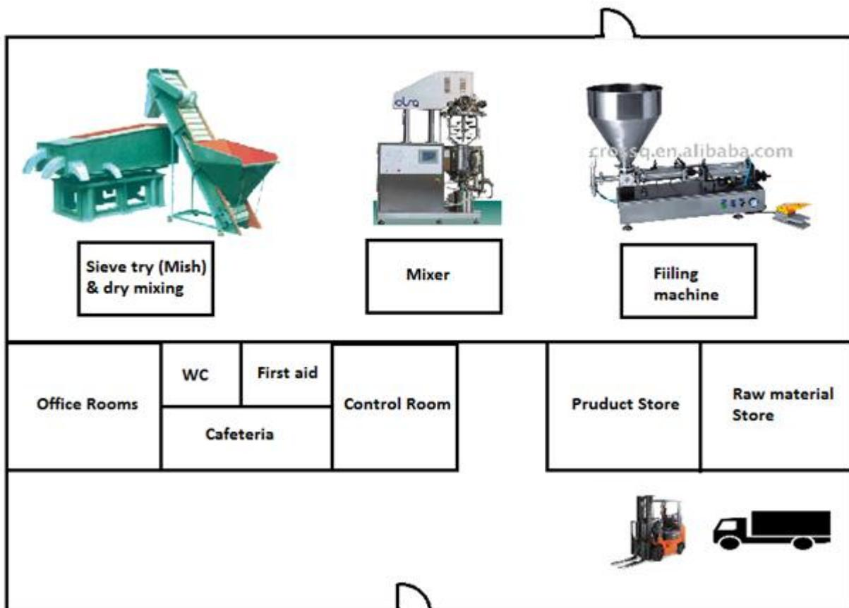
Figure 23: The lay out of the plant.
