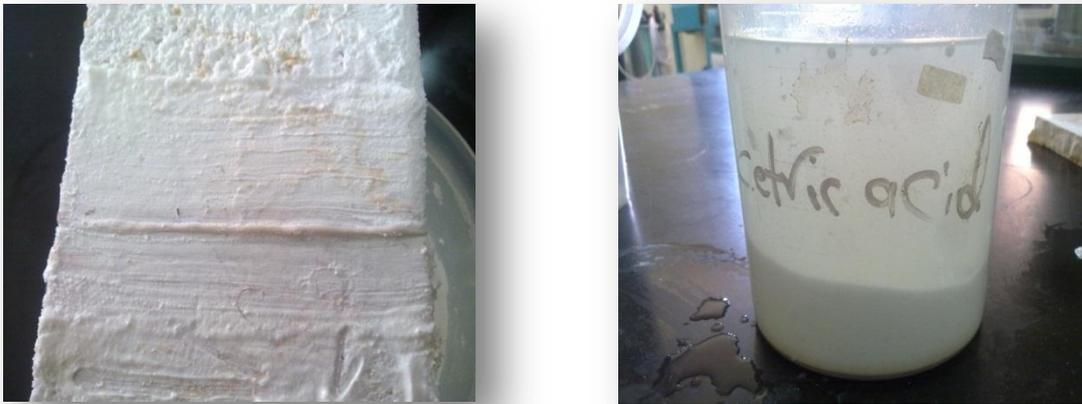
**Figure 14: The sample after soaking in Citric acid.**
