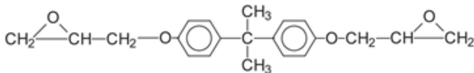
**Figure 5: Epoxy resin**
