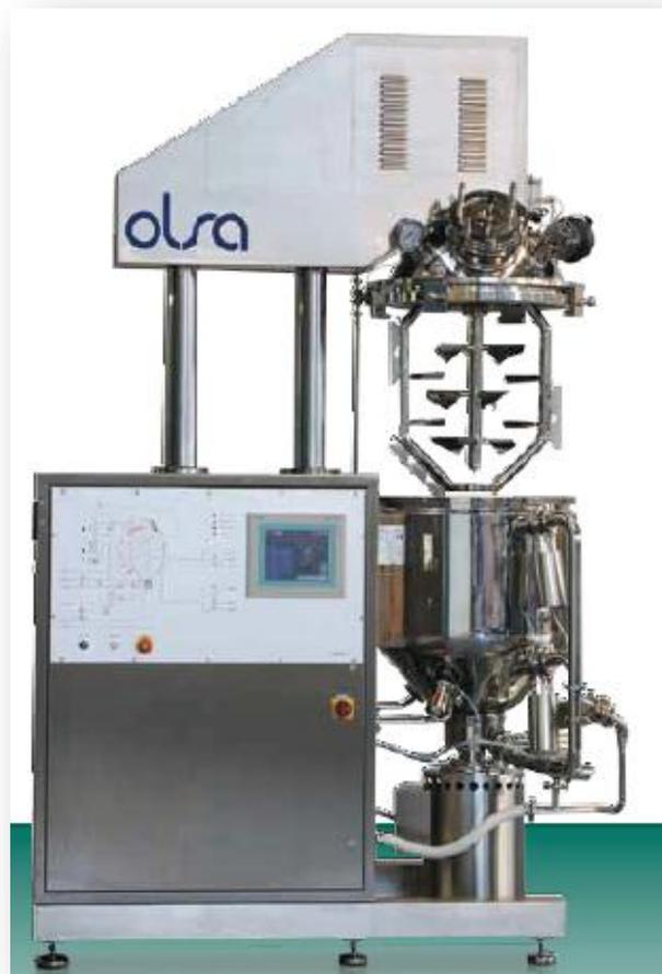
**Figure 24: Speedy mix Vacuum mixer homogenizer [20].**
