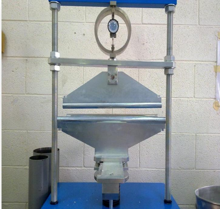
**Figure 8: Flexural machine.**
