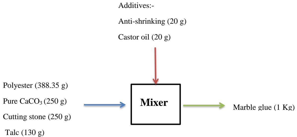
**Figure 20: Flow diagram of raw material.**
