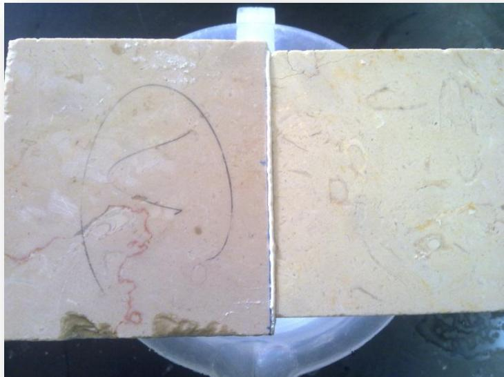
**Figure 16: The sample after soaking in Water.**
