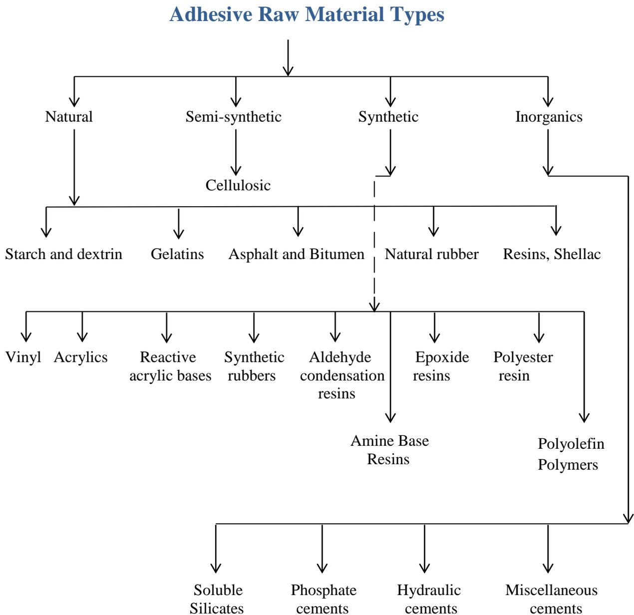
**Figure 1: Adhesive Raw material Types.**
