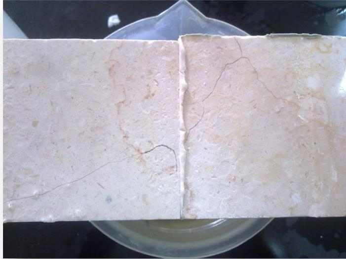
**Figure 15: The sample after soaking in HCl.**
