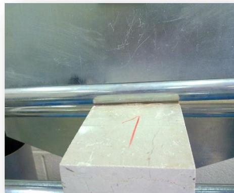
**Figure 10: Fixing the sample on the machine.**
