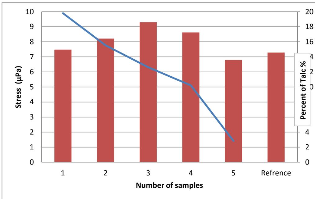
**Figure 19: The stress and the percentage of talc added to the samples.**
