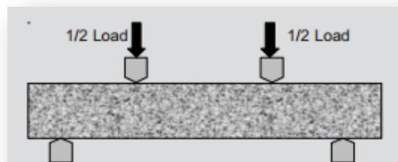
Figure 7: 4-point flexure test.
