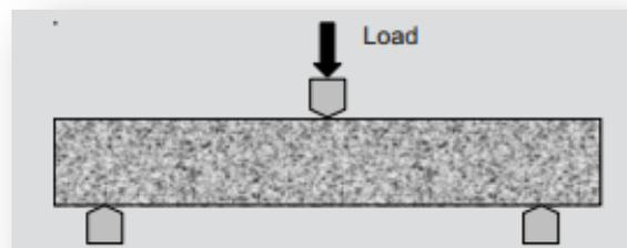
Figure 6: 3-point flexure test.
