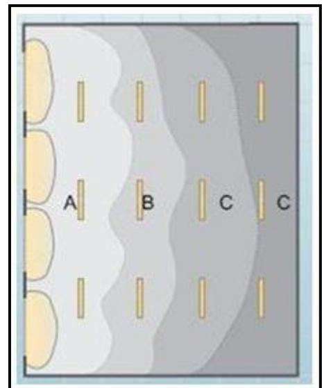
**Fig. 3.9.15** zone of general lighting for daylight harvesting.
