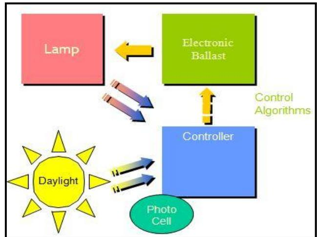
**Fig. 3.9.16** Daylight harvesting control systems.
