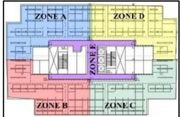
**Fig. 3.9.2** Control zones diagram.
