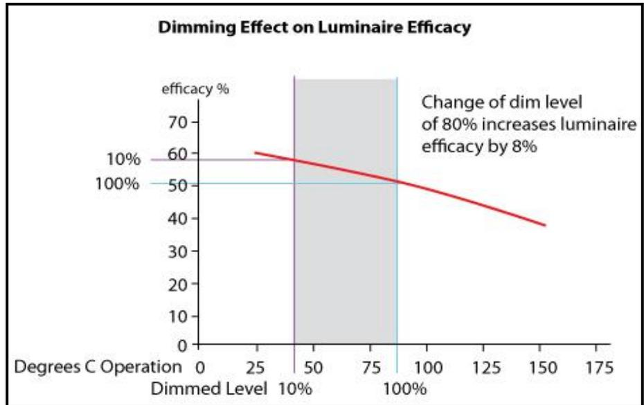
**Fig. 3.9.21** Dimming effect on luminaire efficacy.
