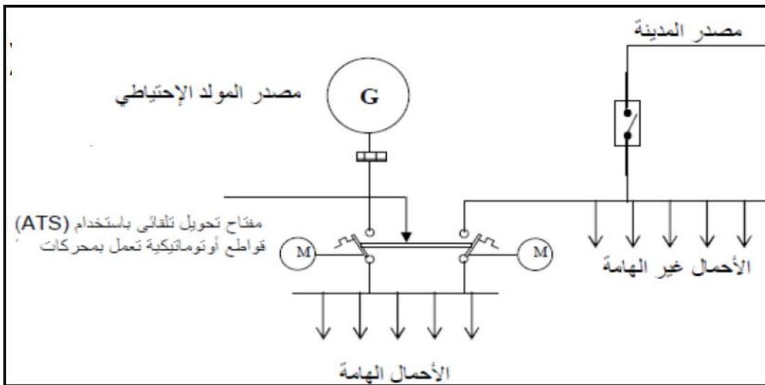
Fig. 3.5.7 Emergency distribution board.
