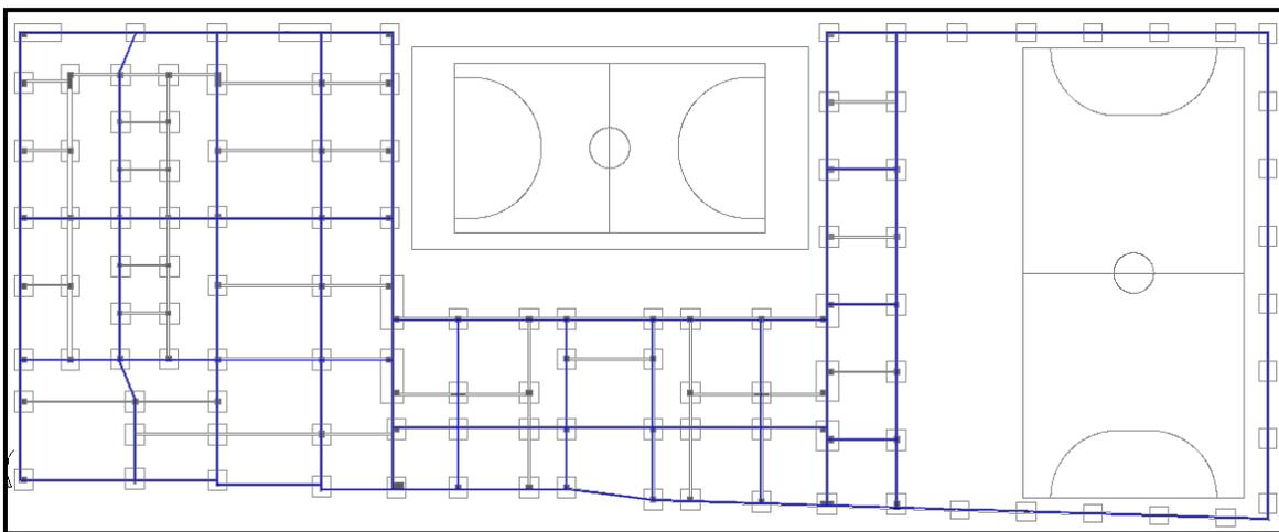
Fig. 3.7.4 Proposed earthing grid
