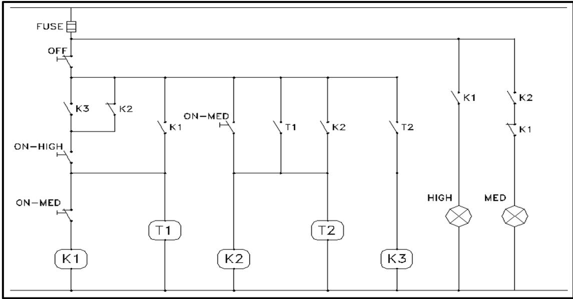
**Fig. 3.6.10** Schematic of control circuit.
