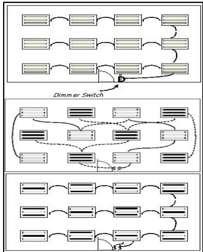
**Fig. 3.9.24** Methods of light level reduction control.
