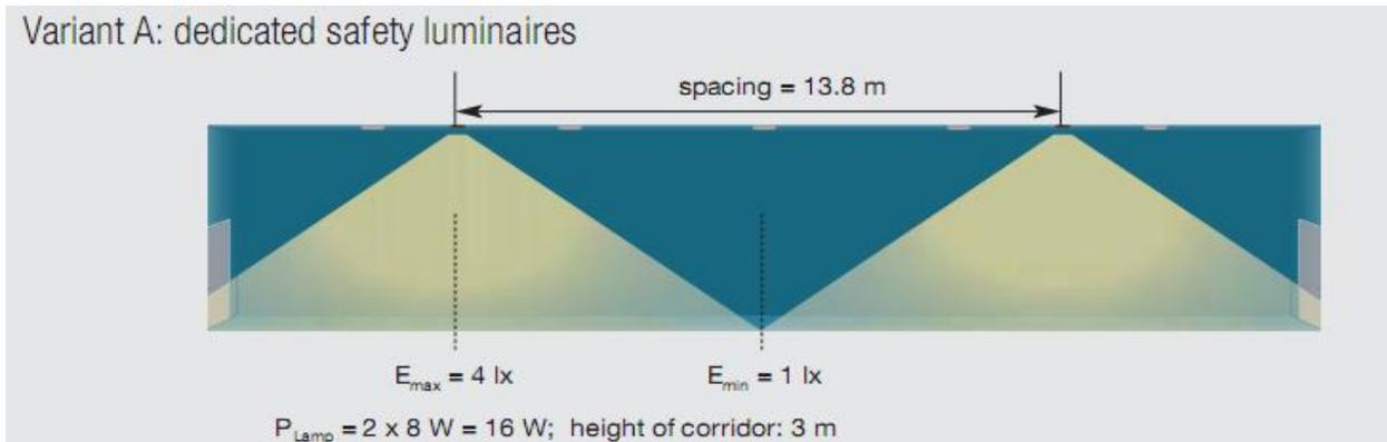
**Fig. 3.5.6** Luminaires for safety lighting modes.
