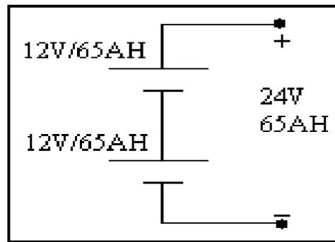
**Fig. 3.5.10** Battery configuration.
