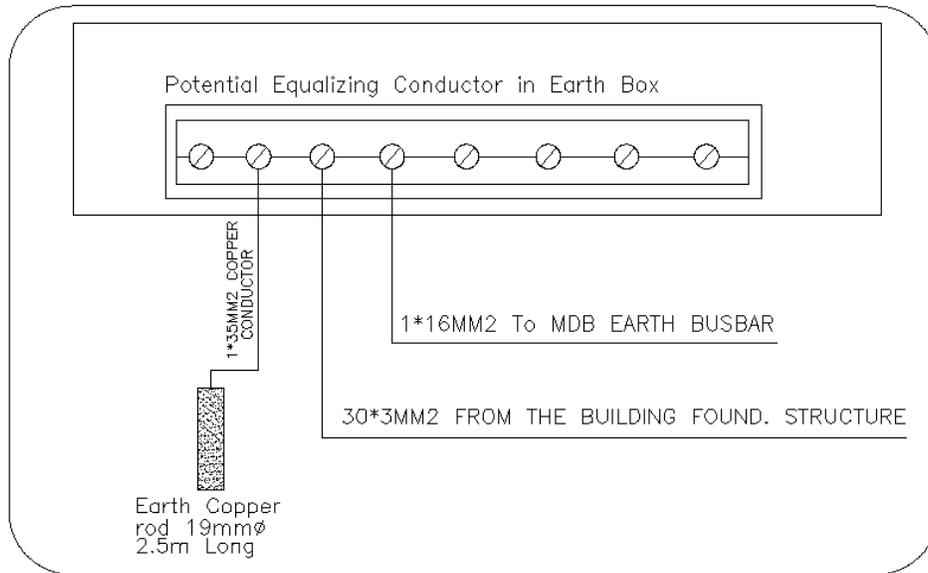
**Fig. 3.7.5** Main Earthing Busbar (MET).
