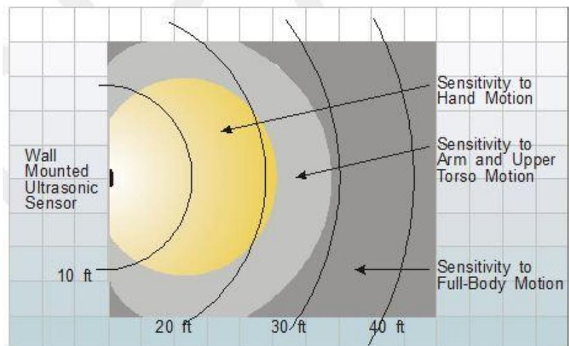
**Fig. 3.9.9** Ultrasonic sensors coverage area.
