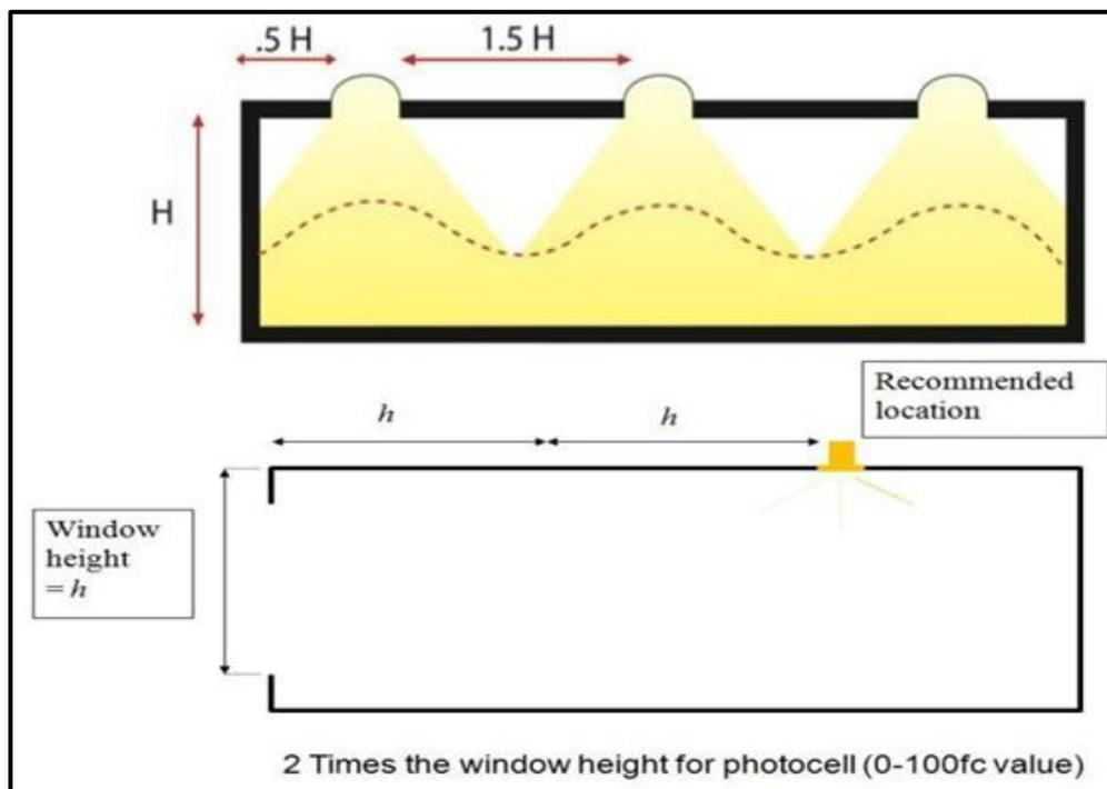
**Fig. 3.9.17** Ideal Applications of daylight harvesting.
