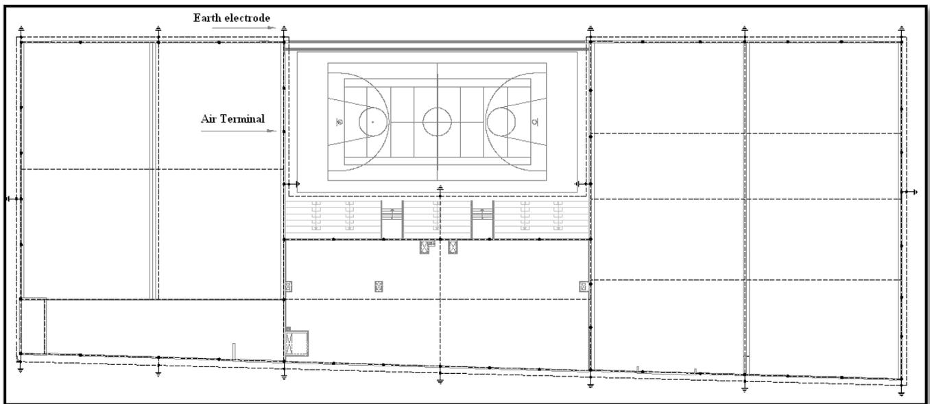
Fig. 3.7.7 The proposed lightning protective system design.
