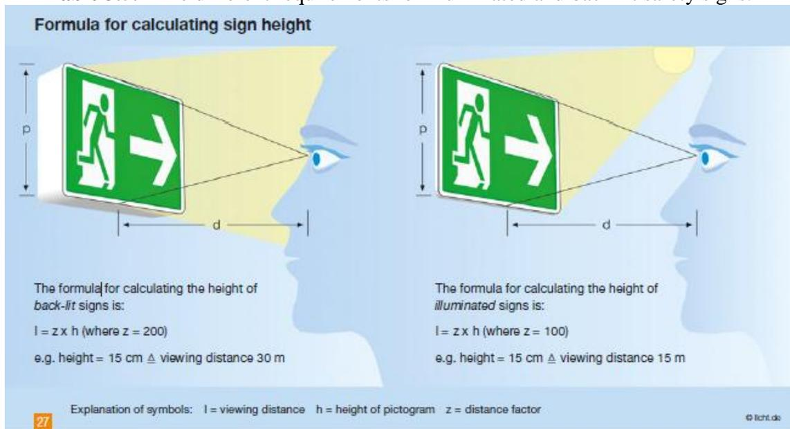
**Fig. 3.5.4** Formula for calculating sign height.
