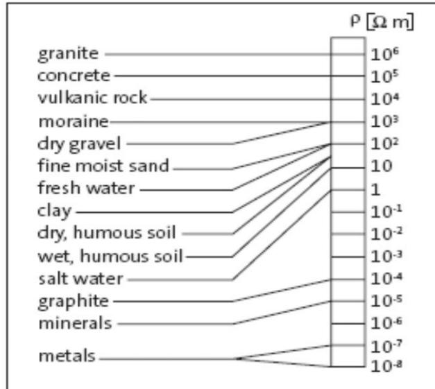
**Fig. 3.7.2** Resistivity in various type of soil.
