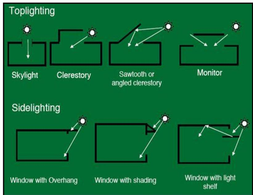
daylight may enter a building via top lighting (e.g., skylight) or side lighting (e.g., window) apertures. Good daylight design enables diffuse daylight to serve as a primary source of general illumination, while avoiding glare and heat gain.
