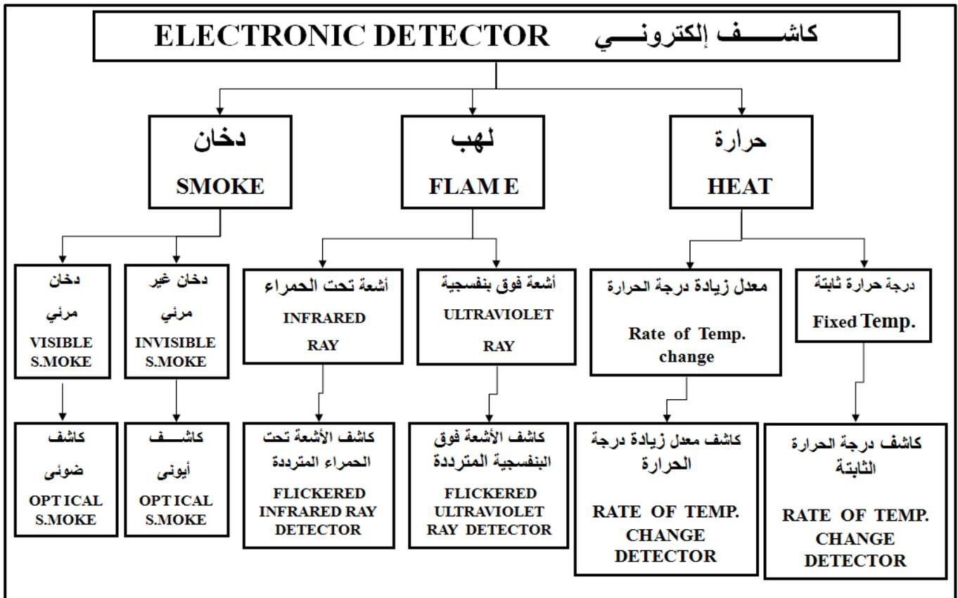
Fig. 3.8.1 Electronic detectors.
