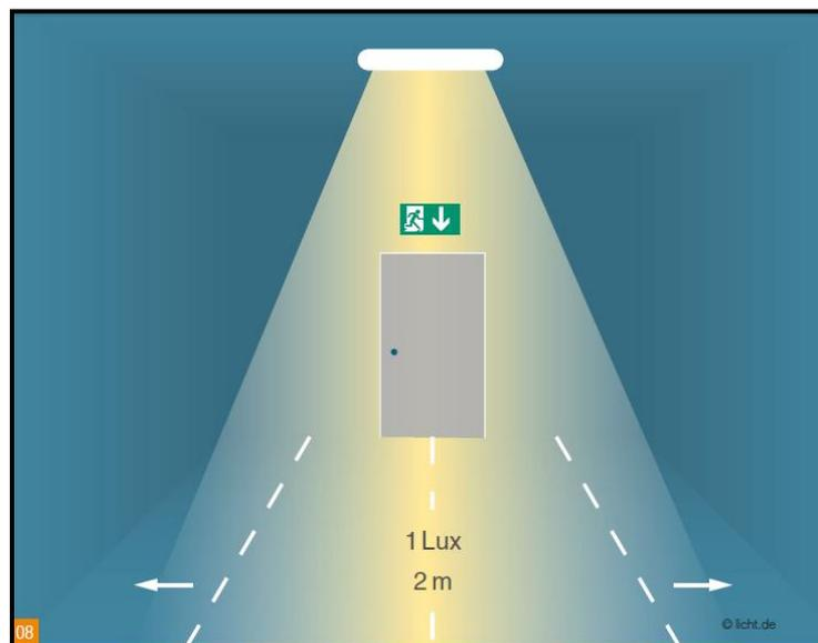
Fig. 3.5.2 Escape route safety lighting specification
