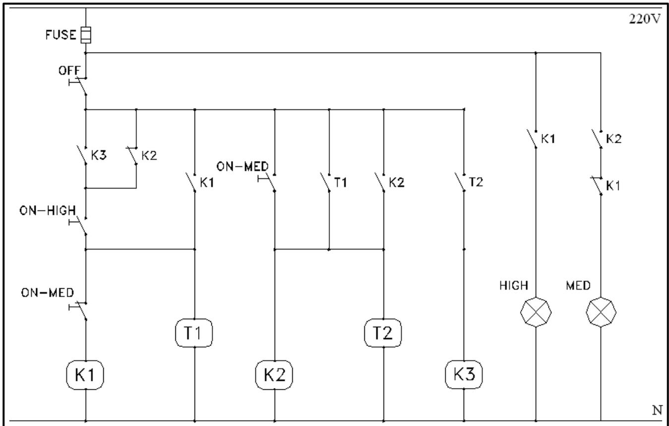
**Fig. 3.6.14** Schematic of control circuit.
