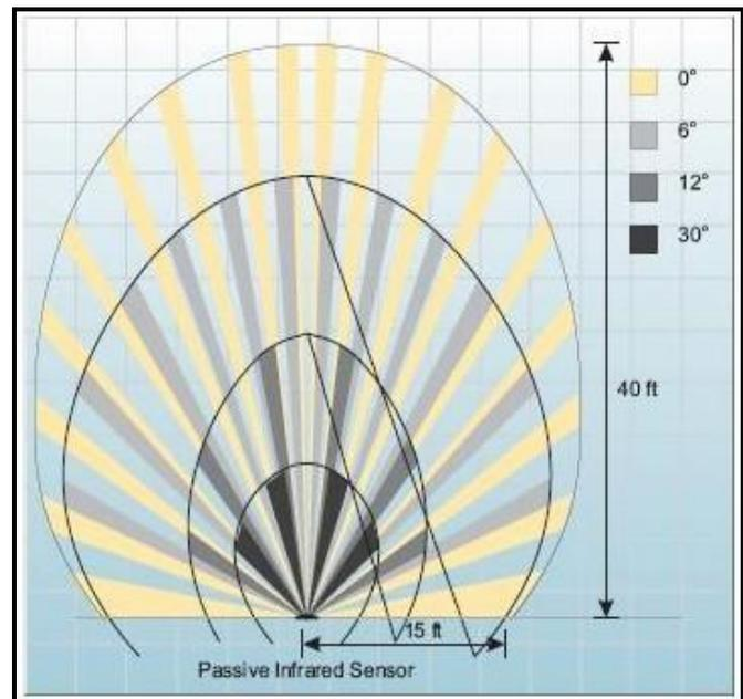
**Fig. 3.9.6** PIR sensors coverage area
