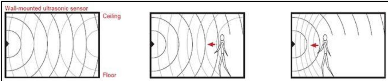
**Fig. 3.9.8** Principle of operation of ultrasonic sensors.
