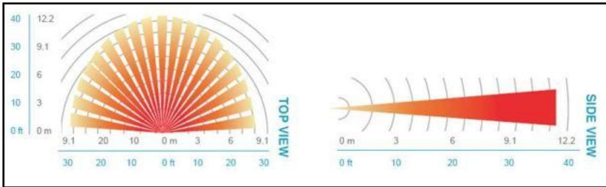
**Fig. 3.9.11** Top & side view of acoustic detection sensors.
