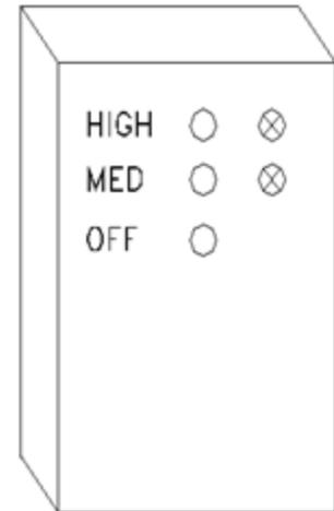
Fig. 3.6.7 Outside appearance of control panel
