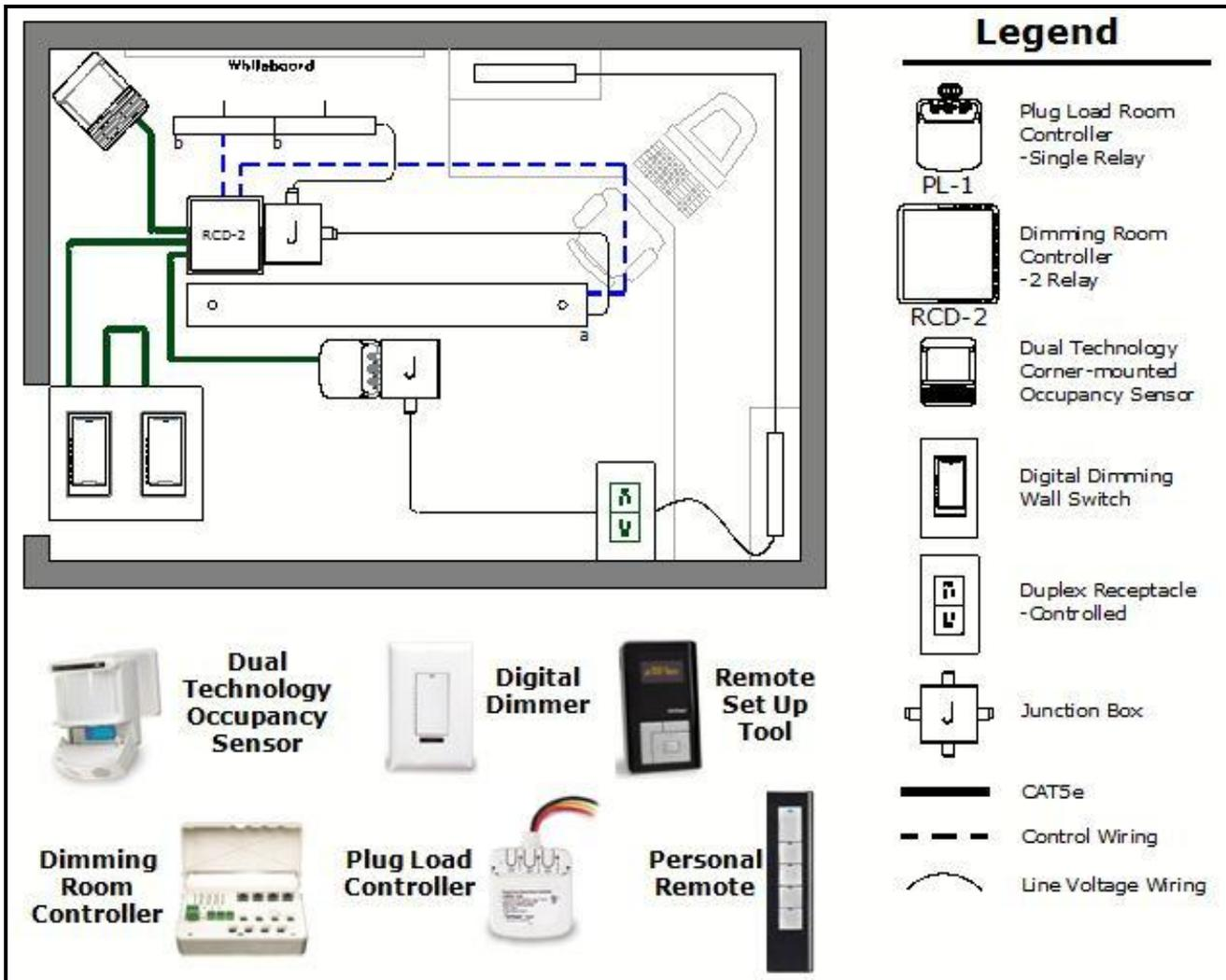
**Fig. 3.9.22** Dimming controller parts.
