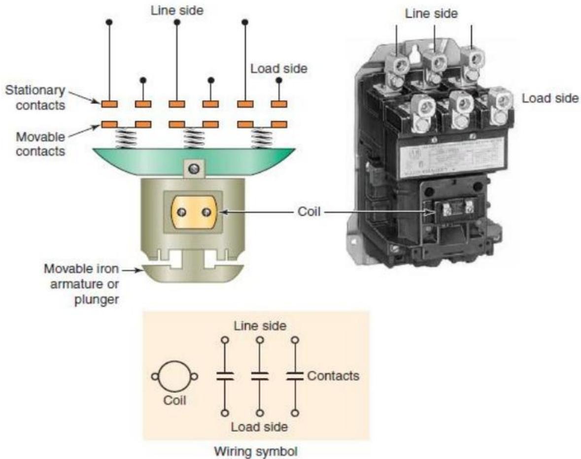
**Fig. 3.6.1** Three-pole magnetic contactor
