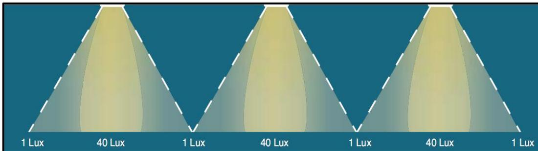
**Fig. 3.5.3** The ratio of the highest to lowest illuminance along the central axis must not exceed 40:1.
