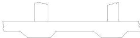
( c ) Flat slab raft thickened under column
